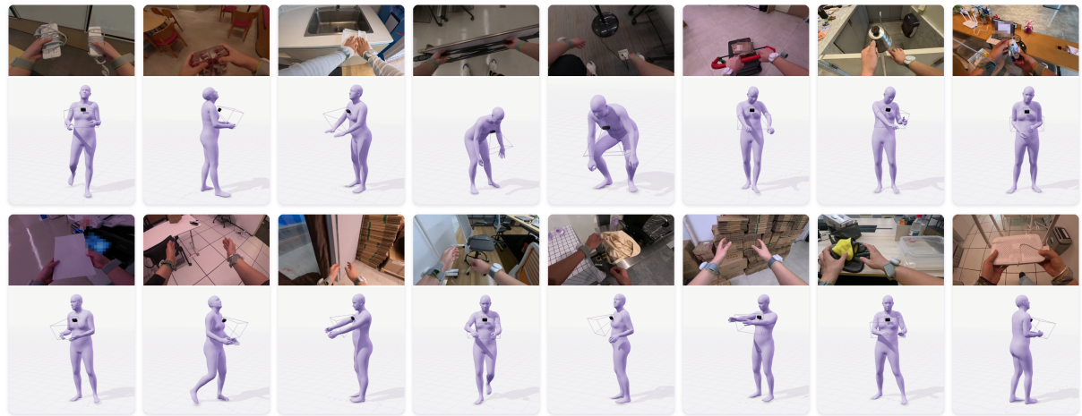
Figure 5: Synchronized human motion and egocentric observations. Top: egocentric RGB frames. Bottom: corresponding SMPL body meshes with MANO hand motion and illustrative camera frusta. Camera frusta schematically illustrate viewing direction.
